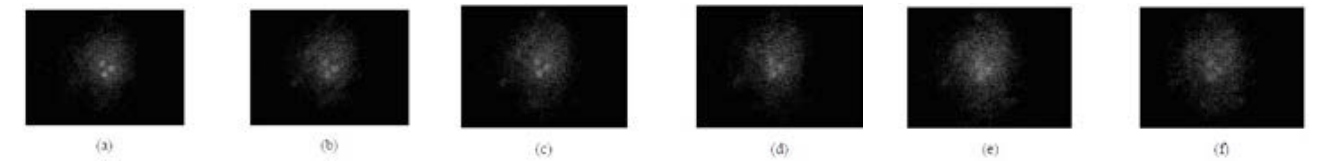
Fig. 3 shows the conjugate signal observed on the CCD. We place the CCD at the difference places to check tolerance of the system including (a) on-focus, (b) 1 mm, (c) 2 mm, (d) 3 mm, (e) 4 mm and (f) 5 mm away from the focus.
