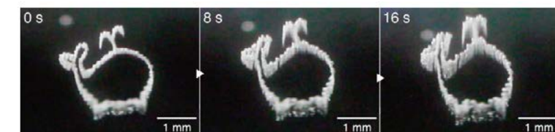
Fig. 3. 2D graphics of "Whale" rendered by femtosecond laser-induced microbubbles.
